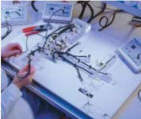
Harness termination on a 3D cabling board with integrated test
